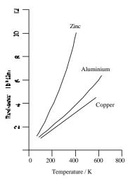
The resistance of a wire at temperature  $T_1$  can be measured with an accurate ohmmeter or calculated with:
