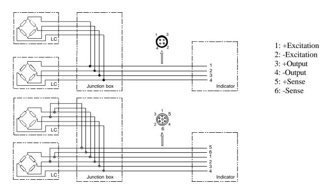
The above figures represent the two basic configurations, using four- or six-wire ( sense ) load cells. With 4-wire extension cables the load cell output should be connected to pairs of diagonally opposite wires.
