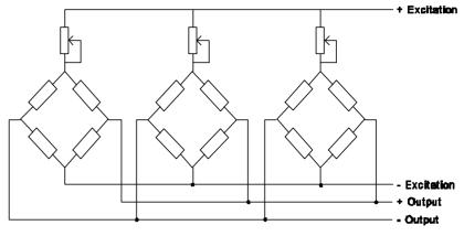
potentiometers by trial and error whilst moving calibration weights around from corner to corner. All potentiometers should be adjusted to have zero ohm resistance at the start of this procedure. Then once the lowest output corner is located, the other cells are trimmed to match this lowest output.
