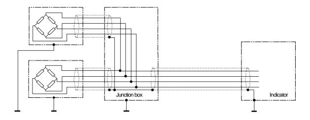
The load cell case and junction box are grounded by mechanical attachment to the structure to which they are mounted. Usually this structure is grounded. The braided shield enclosing the load cell leads is grounded at the indicator, which is grounded through the power cord or housing.
